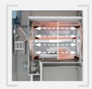
Best drying results No over-drying thanks to Residual Moisture Control (optional) Measures the exact moisture content throughout the whole process
